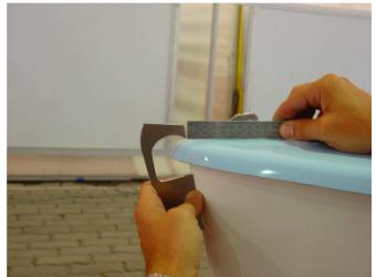
for the forward measurement point (FMP). The length of the hull is given in the measurement form
