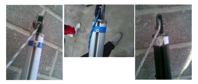
In these examples, the stoppers are positioned for mainsails with square-cut boltrope at the head. In the following picture, you see that if you change into a mainsail with cut-down boltrope, then the stopper for a normal mainsail will not work because the mainsail can be set higher than the limit point. In that case the stopper must be installed in the position shown by the arrow in the following picture:
