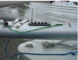
Solution No3: Screw, rivet or other obstacle inside the sail track. This is an easy solution for masts with rope halyards and a clam-cleat.
